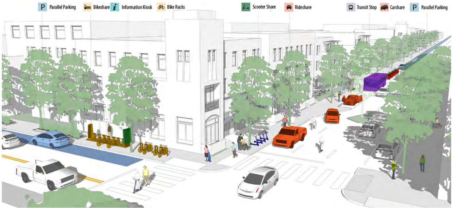
Figure B.15. Mobility Hub at Whittier Boulevard and 4th Street would provide mobility options to residents, employees, and visitors in the Downtown Area and provide connectivity to transit. As shown in the mobility hub illustration, improvements could include providing bus shelters, informational signage, bike parking, and designated loading/unloading curb-space for TNCs.
