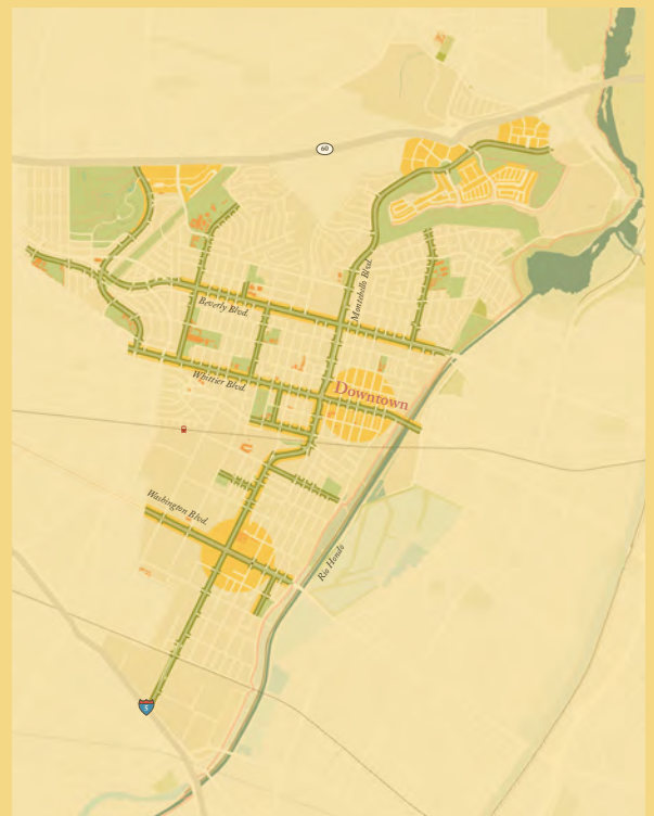
Figure B.1. Key concept map. The General Plan seeks to direct new growth to corridors, the downtown area, future light rail transit stop along Washington Boulevard, and larger tracts along the freeway.
